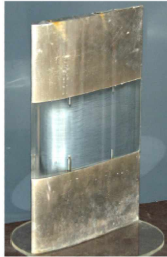
Figure 2.14: A photograph of airfoil SD7003.
