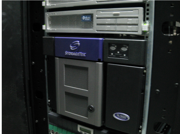
Figure 16. New tape unit employed on ITU-CSCRS ground station
