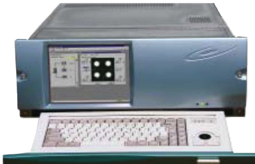
Figure 18. In-Snec software based demodulator system
