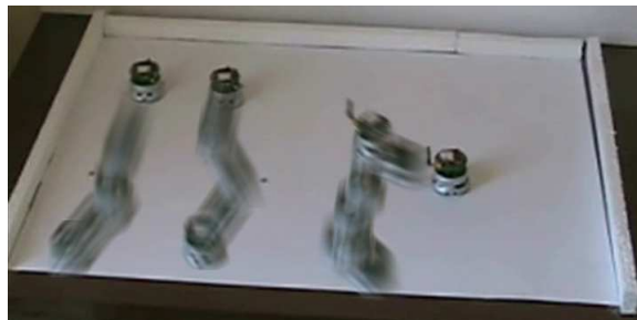
Figure 5.22: Three Khepera II robots divide the labor of visiting the six targets
