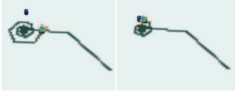
Figure 5.9: An implementation of the Archimedean spiral with the corresponding robot behavior
