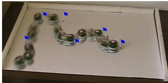
Figure 5.21: The Khepera II robot visits six targets in the environment
