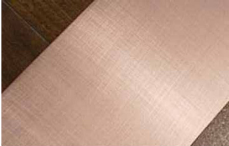
Figure 29 PCB surface after rubbing with abrasive pad
