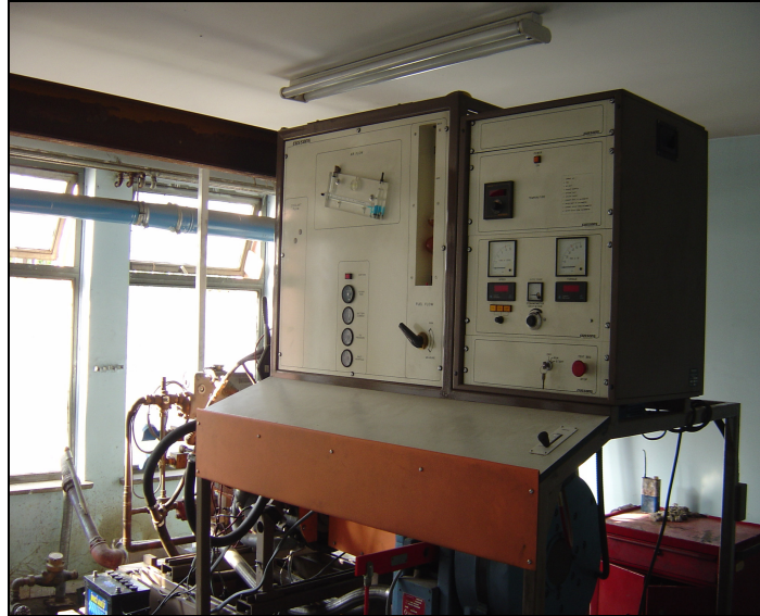
Resim 4.1. P8602 Multi-Cylinder Engine Test dinamometre seti
