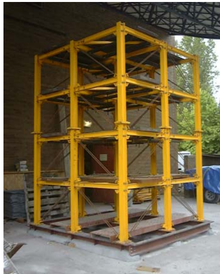
Figure 3.4. The steel frame used for the ASCE SHM benchmark problem (ASCE SHM benchmark website, 2006)
