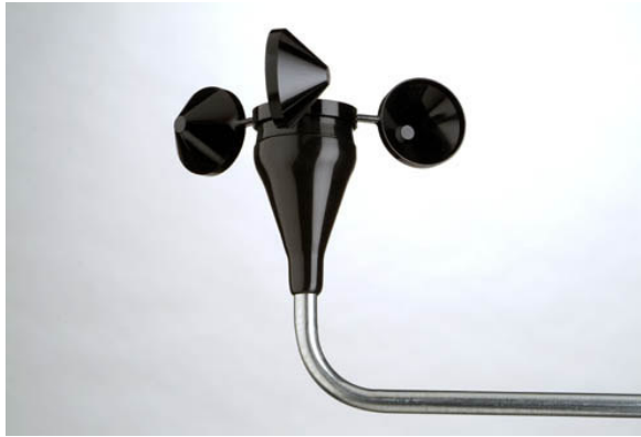
Figure 2.11 NRG maximum #40 cup anemometer
