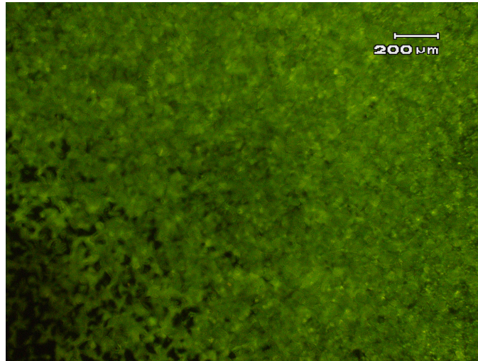
Figure 3.12 Attached cells on the 20 W 15 minute plasma applied PMMA surface.
