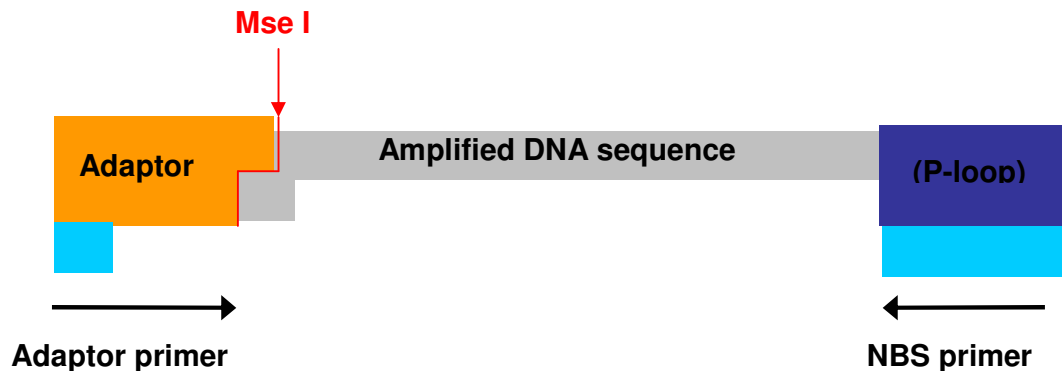
Figure 1.7. NBS-profiling technique targets DNA sequences between conserved NBS motifs and restriction enzyme cut sites ( Mse I in this case).
