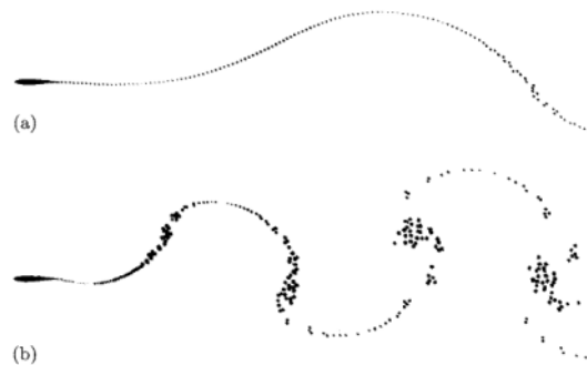
Figure 1.10 : Computed vortical wake due to sinusoidal plunging motion (a) k = 0.5 , (b) k = 1.0 (adopted from Cebeci et al., 2005).
