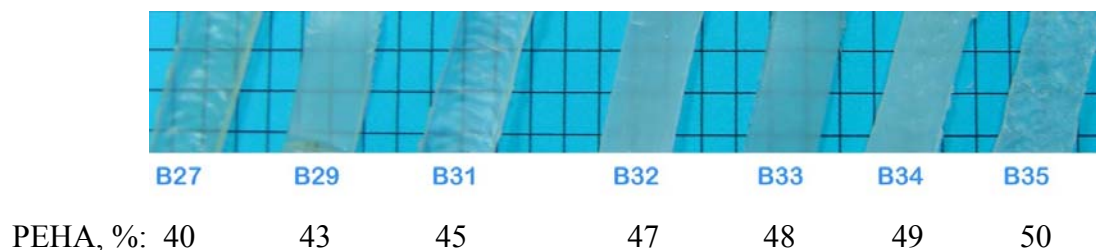
Figure 4.86 : The strip film images of PS- b -PEHA- b -PS baroplastic tri-block copolymers (PEHA%,40-50, B27-35) in different compositions obtained by extrusion process.
