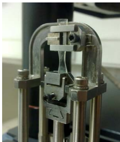
Figure 4.87 : The measured strip film images of PS- b -PEHA- b -PS (40% PEHA, B27) baroplastic tri-block copolymers by DMA.
