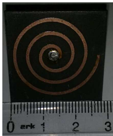
Figure 4.2 Front section of fabricated model of CSMPA 2.8x2.8 cm
