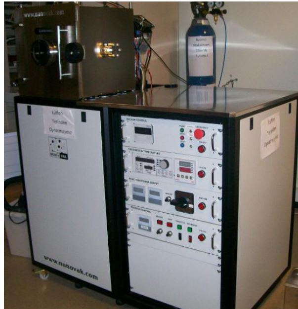
Figure 4.30: The evaporator coating system in our laboratory
