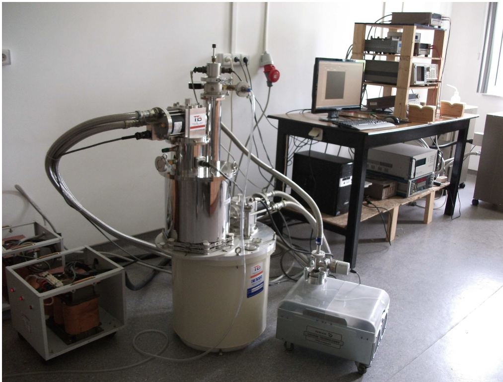
Figure 2.4: He gas contact cryocooler and superconducting coil magnet from CRY Industries.
