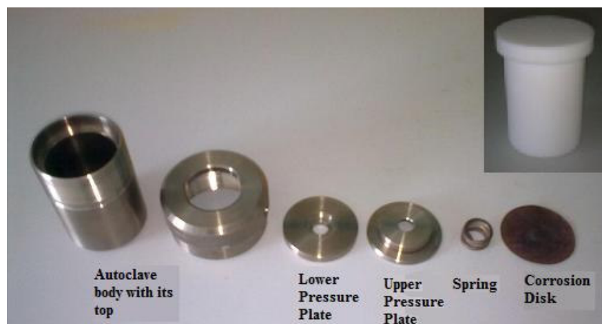
Figure 2.1. Schematic representation of an autoclave with its parts. (Inset shows the Teflon liner) (Source: Kepenekci, 2009)
