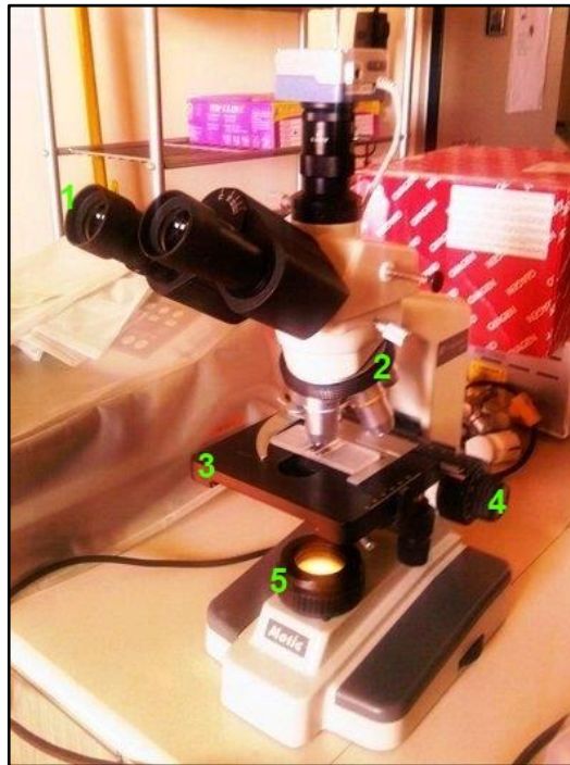
Figure 4. Light Microscopy essential parts
