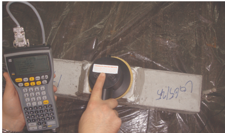
Figure 3.13. Testing with the Galvapulse device.
