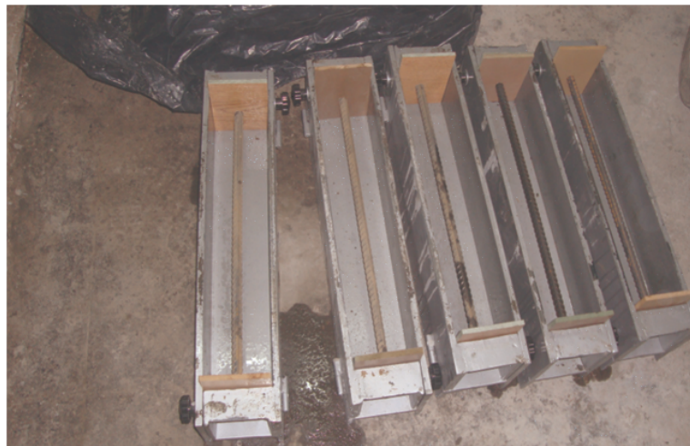
Figure 3.2. Replacement of the steel rebar into the steel mold.
