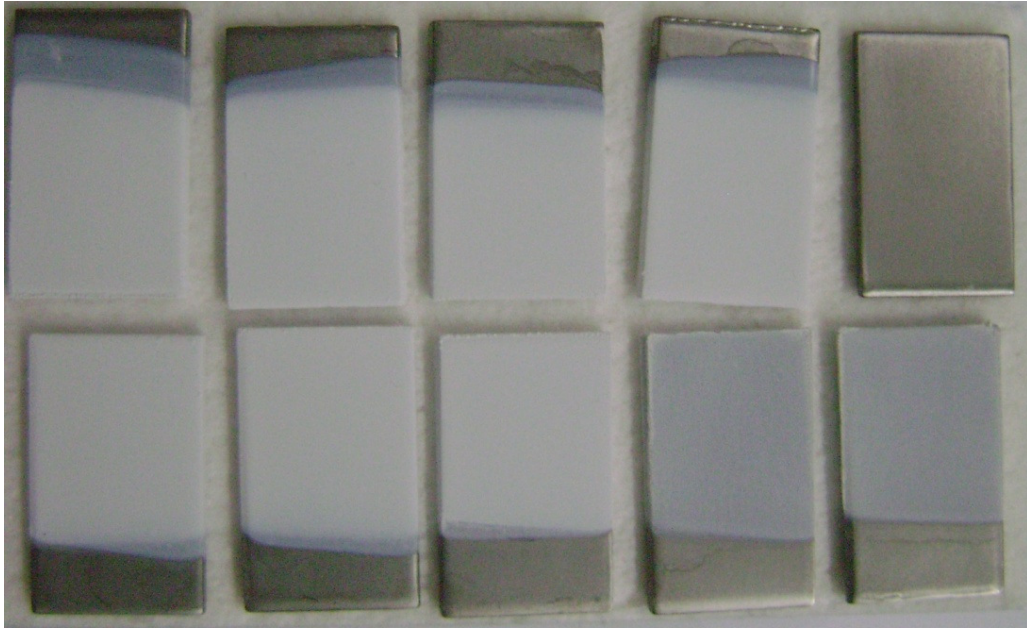
Figure 3.6. XRD samples prepared to determine the effects of TiO 2 coating voltage and sintering temperature on 9SHA decomposition (light grey areas: TiO 2 coating; white areas: 9SHA coating; right most sample in the upper row: titanium substrate without coating).
