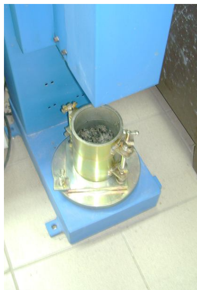
Figure 5.7 Cylindrical mold on compaction equipment
