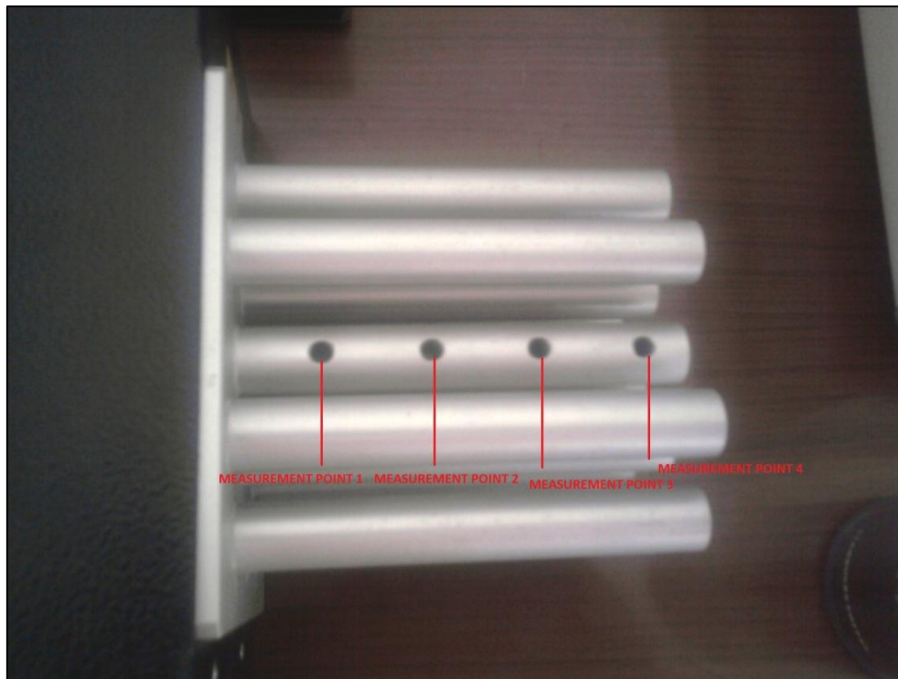
Figure 2.2 Measurement points of Free/Forced Convection Unit for Pipe Bundles
