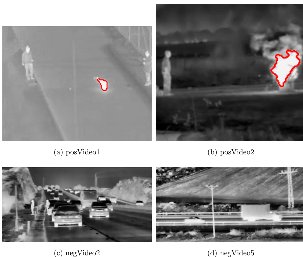
Figure 3.9: Some IR image example results of our IR video flame detection algorithm.
