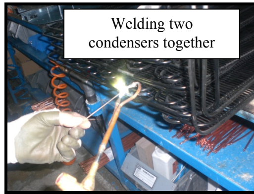
Figure 3.17 Photo of welding operation
