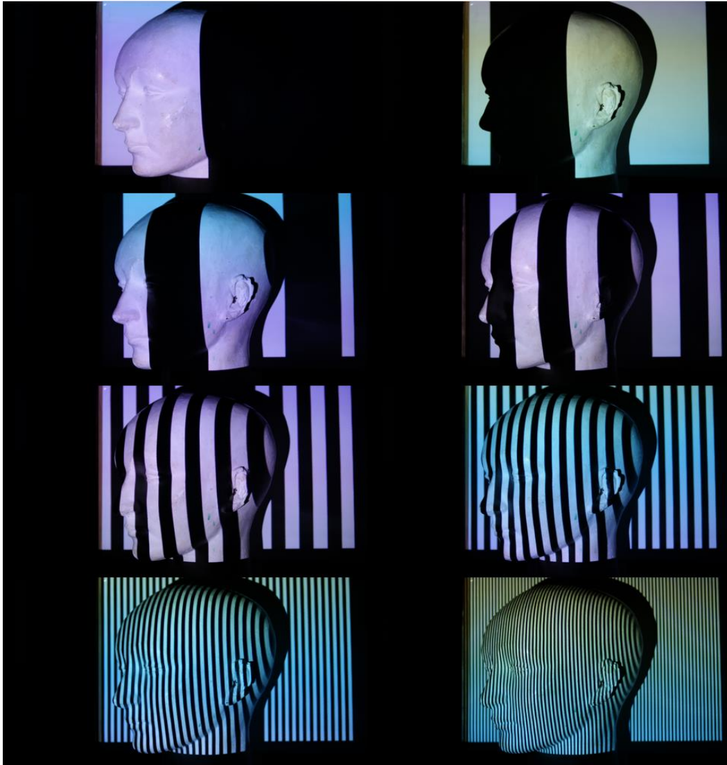
Figure 4.4 Binary pattern projected on a mannequin sequentially with 2^n stripes. n = 8 for our case.
