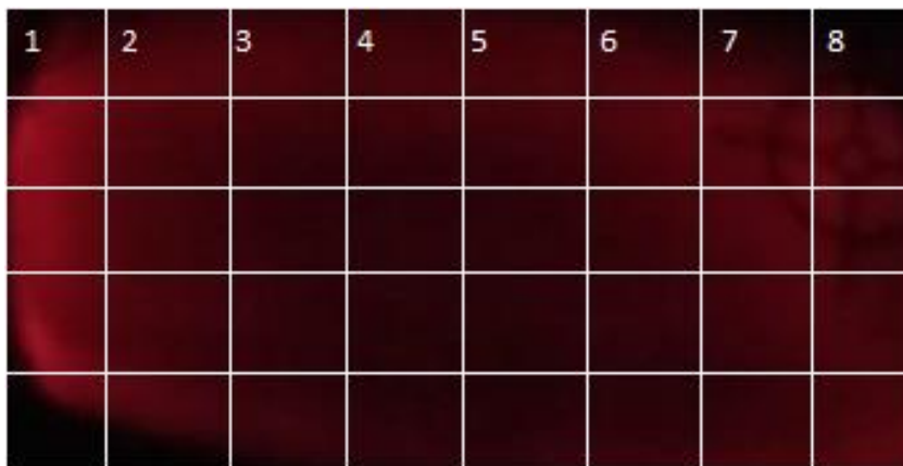
Figure 3.12. b. Portioned laser beam intensity on IR card after DMD.
