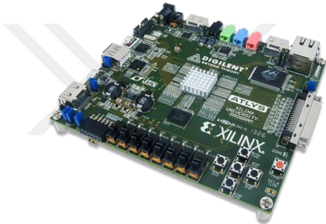
Figure 3.11. FPGA Spartan-6 Family XC6SLX45 Packed CSG324C
