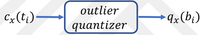
Figure 3.2: In the second stage of pre-preprocessing, discontinuities in the convolved phase c_x(t_i) are detected by using Recursive Least Squares (RLS) algorithm and then quantized to form the vector q_x(b_i) .
