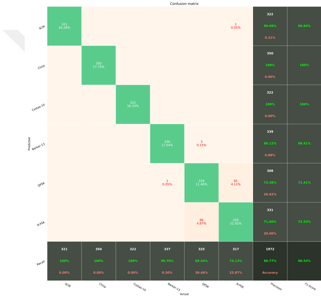
Figure 4.8: Confusion matrix of the WVTFI technique for test data of 6 class set at 10 dB SNR level.
