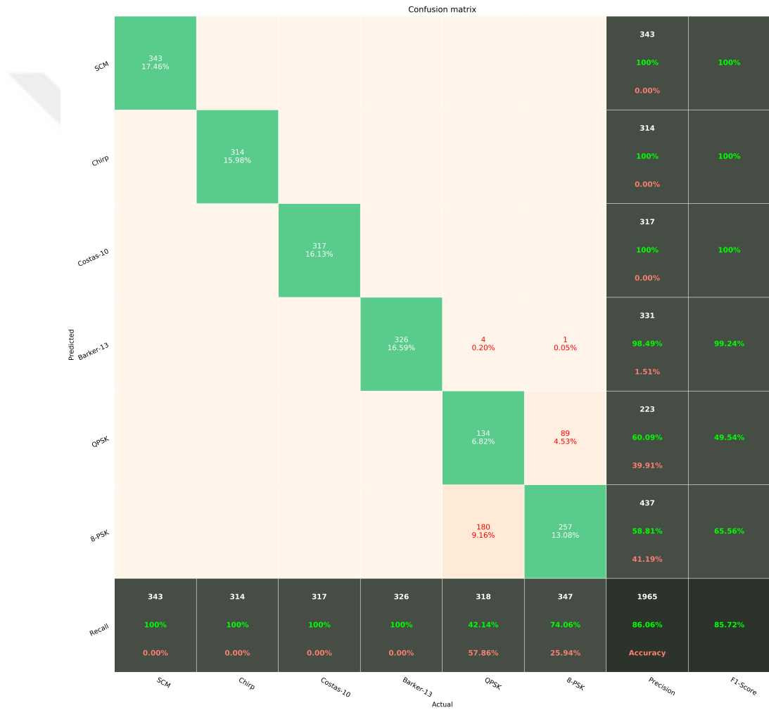
Figure 4.6: Confusion matrix of the pure CNN based model for test data of 6 class set at 10 dB SNR level.
