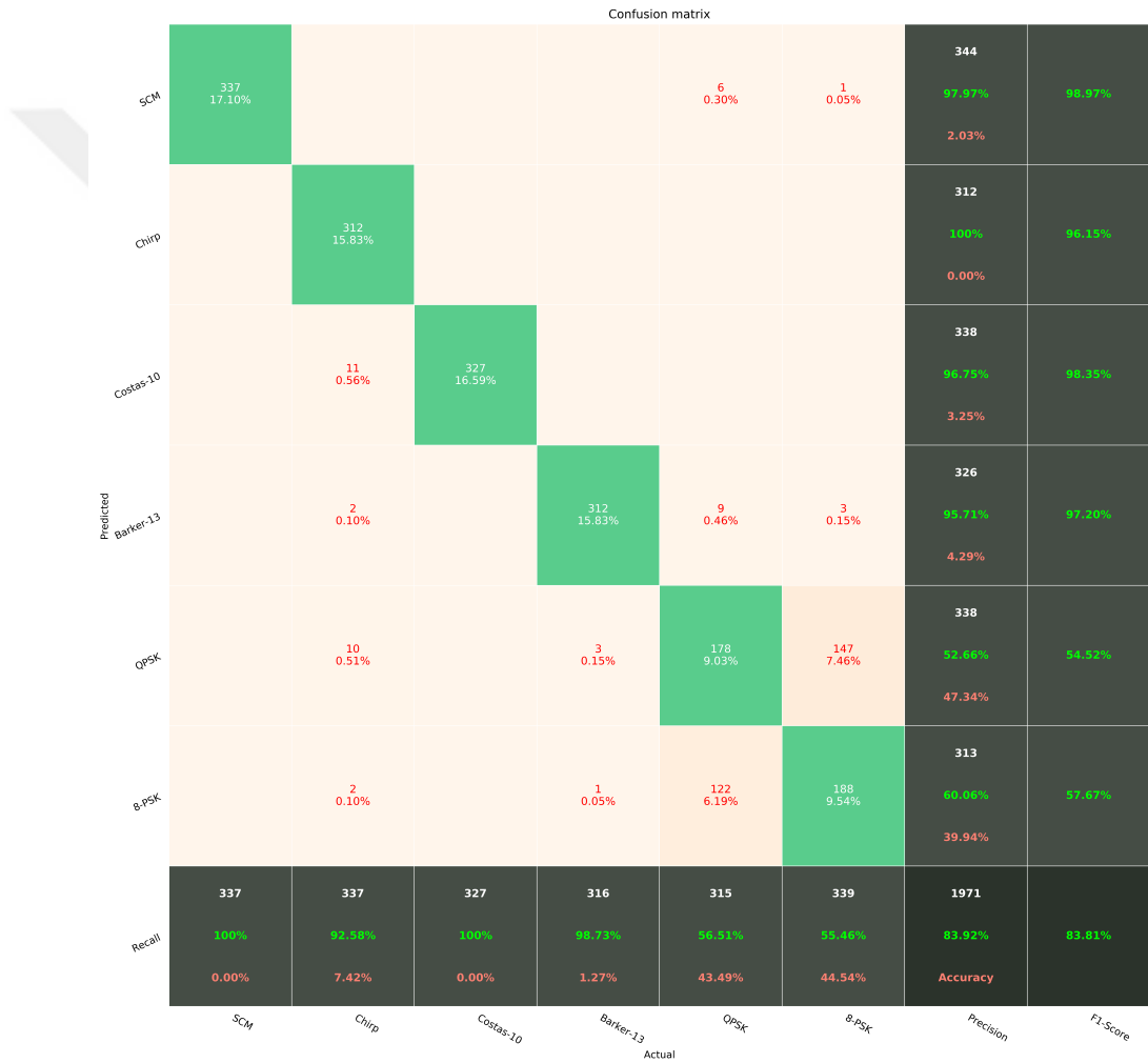
Figure 4.7: Confusion matrix of the pure CNN based model for test data of 6 class set at -10 dB SNR level.
