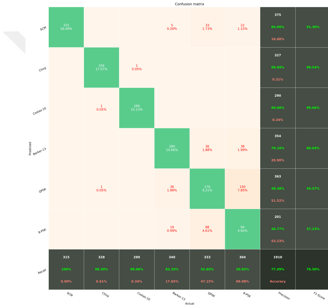
Figure 4.11: Confusion matrix of the CWTFI technique for test data of 6 class set at -10 dB SNR level.
