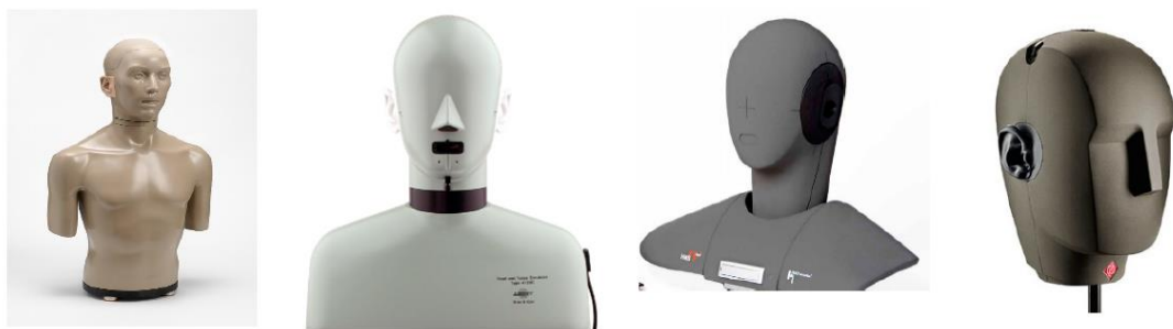
Figure 4. Artificial head (from left to right): KEMAR, Brüel & Kjaer 4128HATS, Head Acoustics HMS III, and Neumann KU-100, (Hong et al., 2017)
