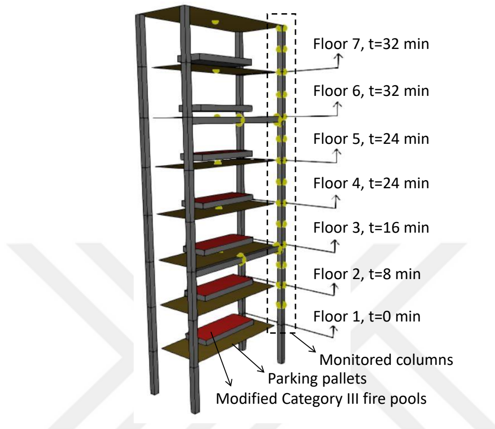
Figure 4.14 Simulation setup for vertical fire spreading
