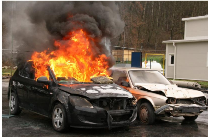
Figure 2.1 Fire test setup lateral fire spreading retrieved from Weisenpacker et al. (2016)
