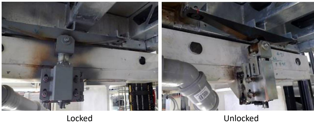
Figure 3.15 An example of parking pallet locking mechanism under the pallet and parallel to the rail (Hrabovský et al. 2019)
