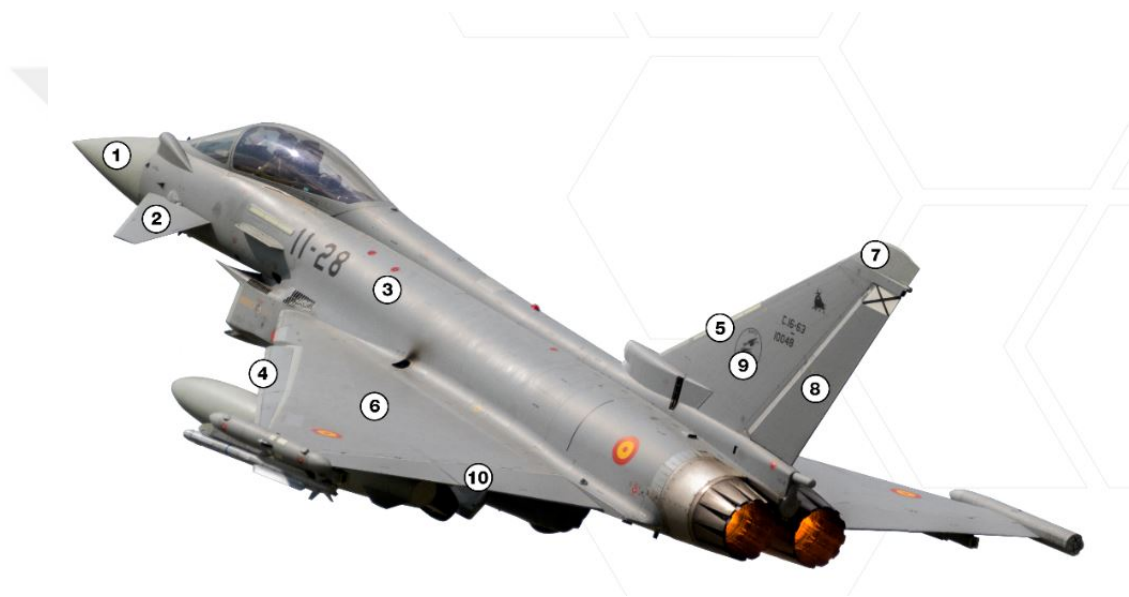
Figure 3.9: The Composite Parts of A Jet Aircraft [6]
