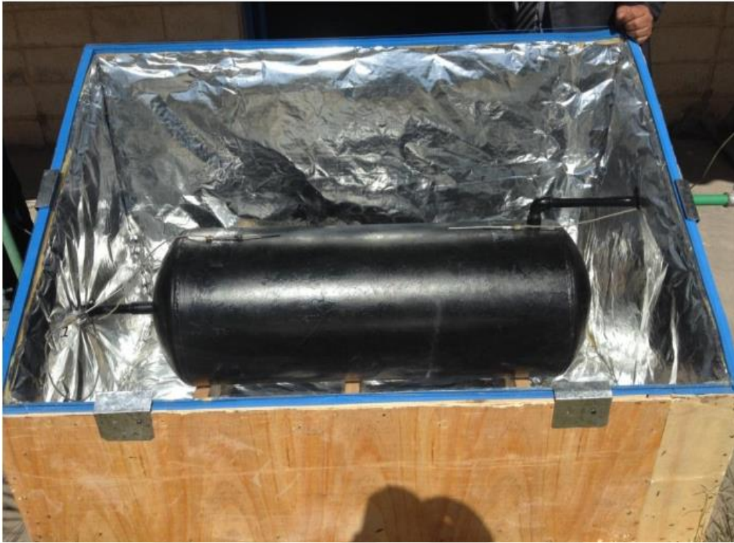
Figure 2.3. Assembling cylinder of solar water heater (Al-shamkhi, 2016).
