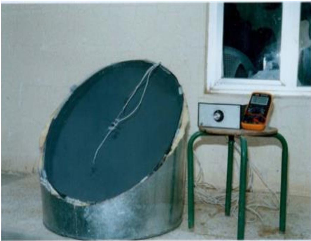
Figure 2.4. Cylindrical storage collector (O.K.Ahmed, 2017).
