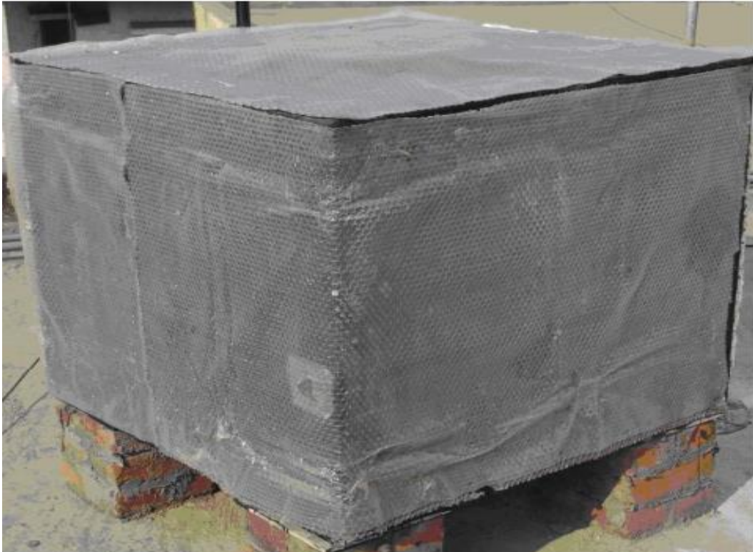
Figure 2.10. Front view of the integrated collector storage solar water heater. (Atish, 2013).
