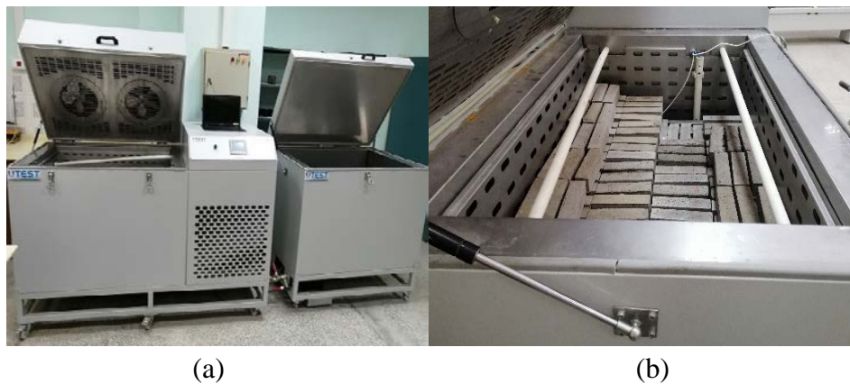
Figure 3.7. Photographic display of freeze-thaw testing: (a) cabin and (b) sampl
