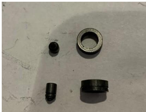
Figure 2.11. Active and passive electrodes made of graphite material for use in EC-08 cell.
