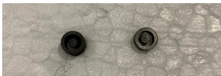
Figure 2.13. Passive electrodes are centered with respect to active electrodes.
