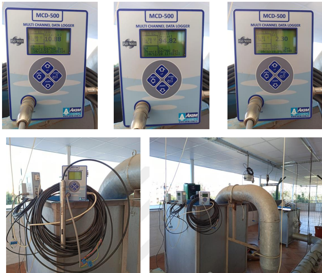
Figure 3.10. The prototype sensor that was put into the test pool and the data logger it is connected to.
