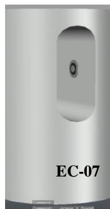
Figure 2.5. Autocad drawing of EC-07. The first design in which active and passive electrodes face each other.
