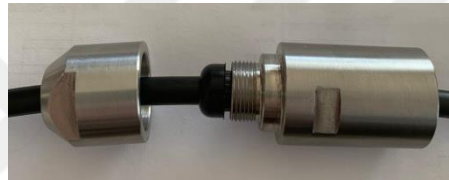
Figure 2.19. The gasket used at the main cable connection point. Thanks to this gasket, both sealing is provided and the load does not get on the cable connection point.
