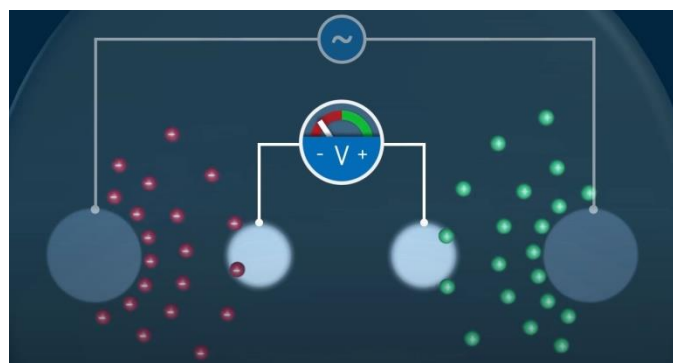
Figure 1.6. Four electrode conductivity measurement (Digital 4-electrode conductivity sensor)
