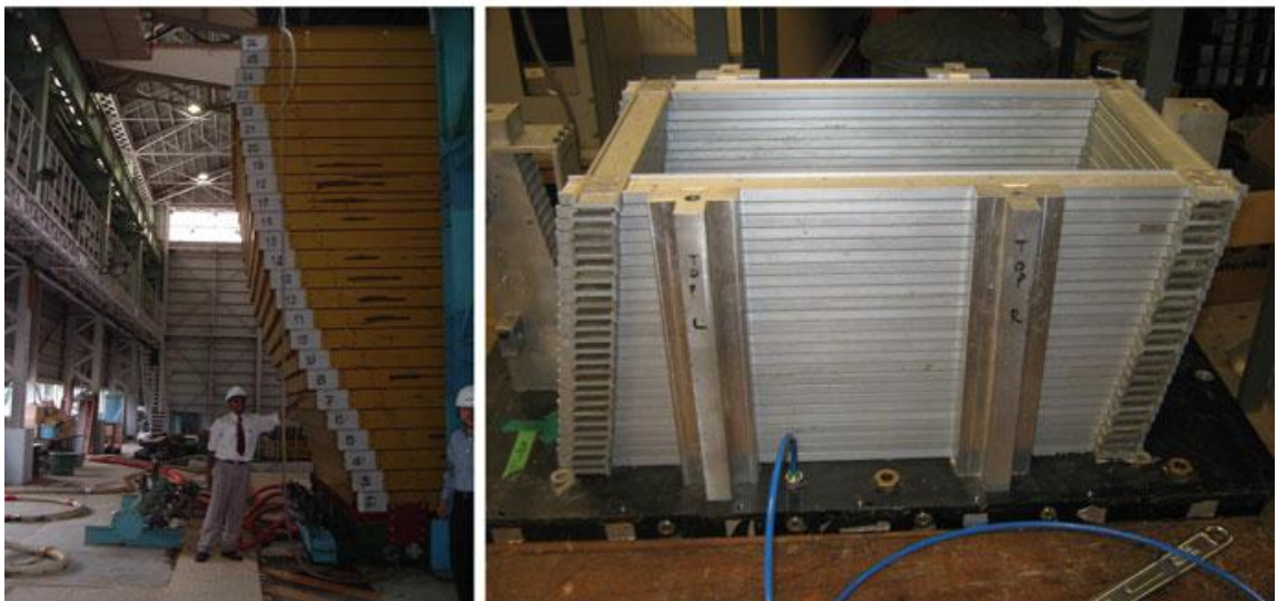
Figure 2.28. Laminar container examples: Large laminar container used in 1-g testing in Tsukuba, Japan (left); Laminar container used in centrifuge, University of Cambridge (right) (Bhattacharya et al. , 2012).
