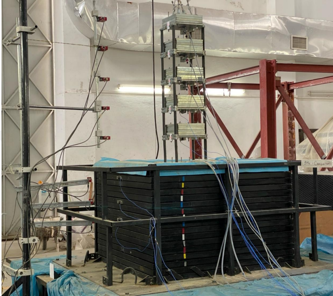
Figure 3.20. Instrumentations of the test model, laminar box and shaking table.
