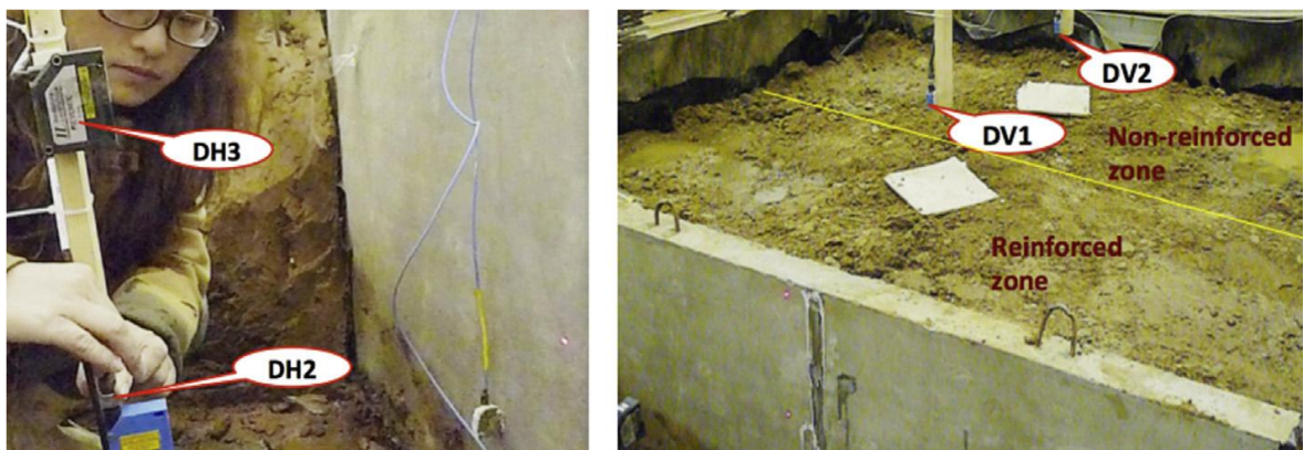
Figure 2.12. Installation of laser displacement meters (Wang et al. , 2015).
