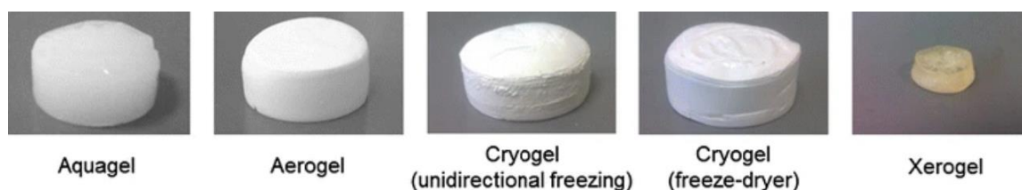
Figure 1.3.3. Examples of cellulose gels after drying with different methods (Reprinted with permission from Springer Nature, Copyright 2020.) [84]
