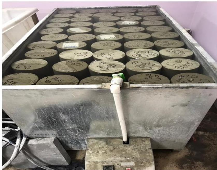
Figure 3.10. Curing basin, the specimens kept 7 days in the tank at temperature 22°.
