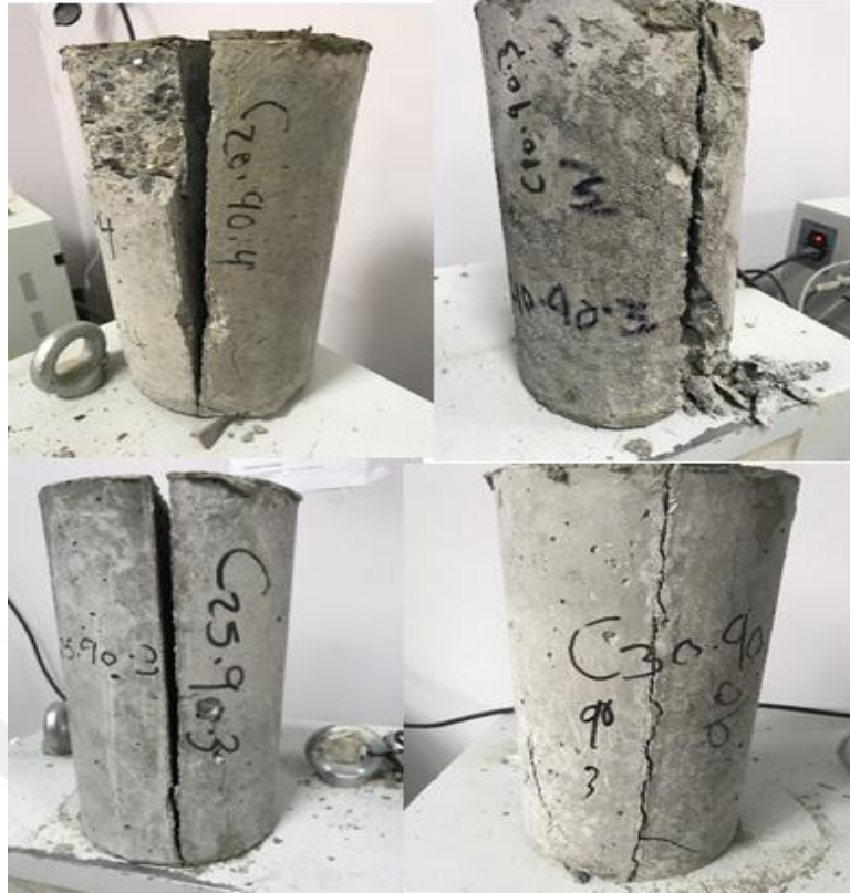
Figure 4.4. Compression test pictures of 90° cold joints.
