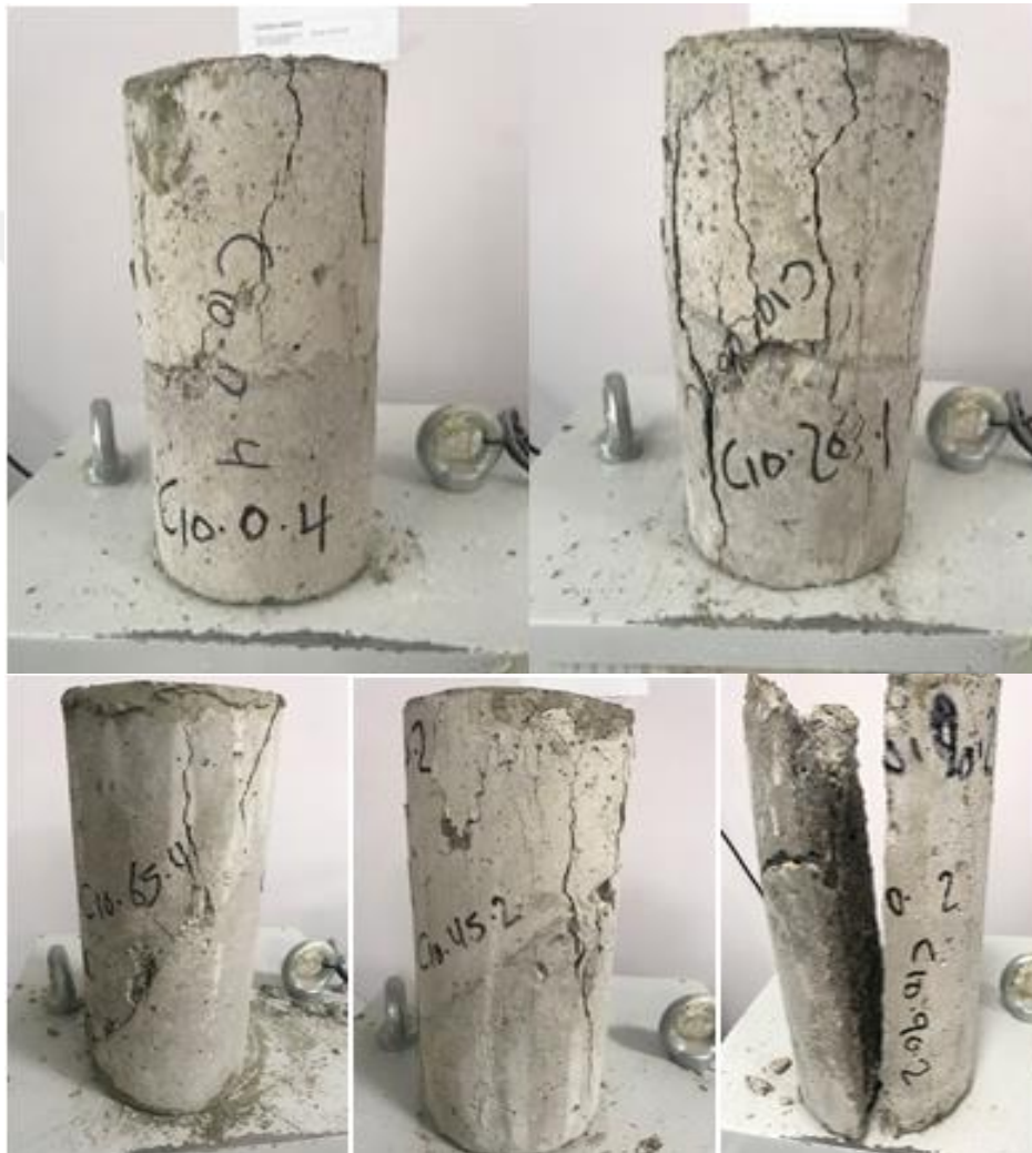
Figure 4.12. Test pictures of samples for 10 MPa strength with different angles.
