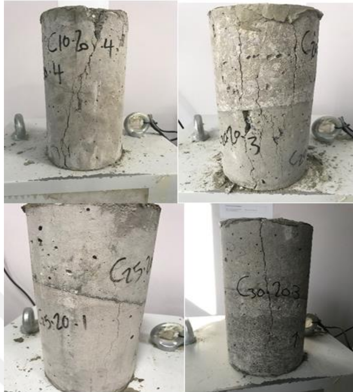
Figure (4.8) Compression test pictures of 20° cold joints.
