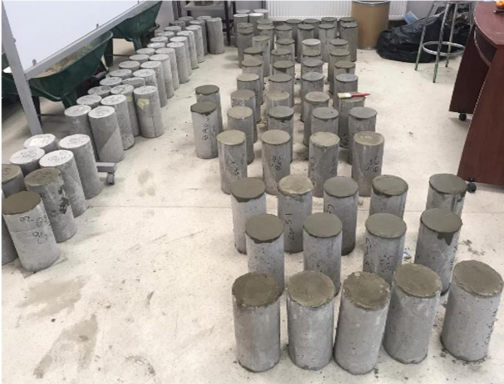
Figure 3.12. Caping the lower and upper surfaces of samples.
