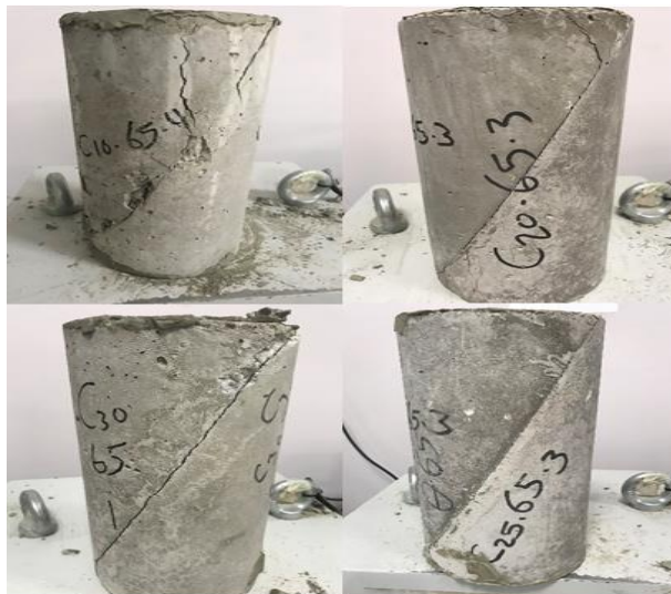
Figure 4.6. Compression test pictures of 65° cold joints.
