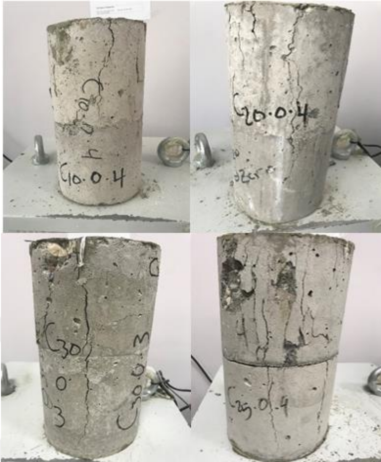
Figure 4.2. Compression test pictures of 0° cold joints.
