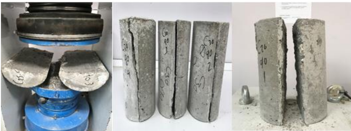
Figure 4.19. Splitting tensile tests for 20, 25 and 30 MPa with 90^\circ cold joint angle.
