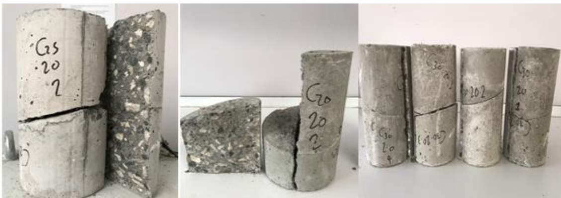
Figure 4.20. Splitting tensile tests for 20, 25 and 30 MPa with 20^\circ cold joint angle.
