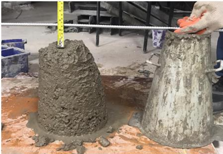
Figure 3.9. The slump test.
