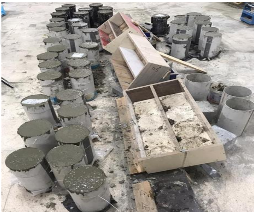
Figure 3.6. The inclination of the base under the mold and the molds after finishing casting.
