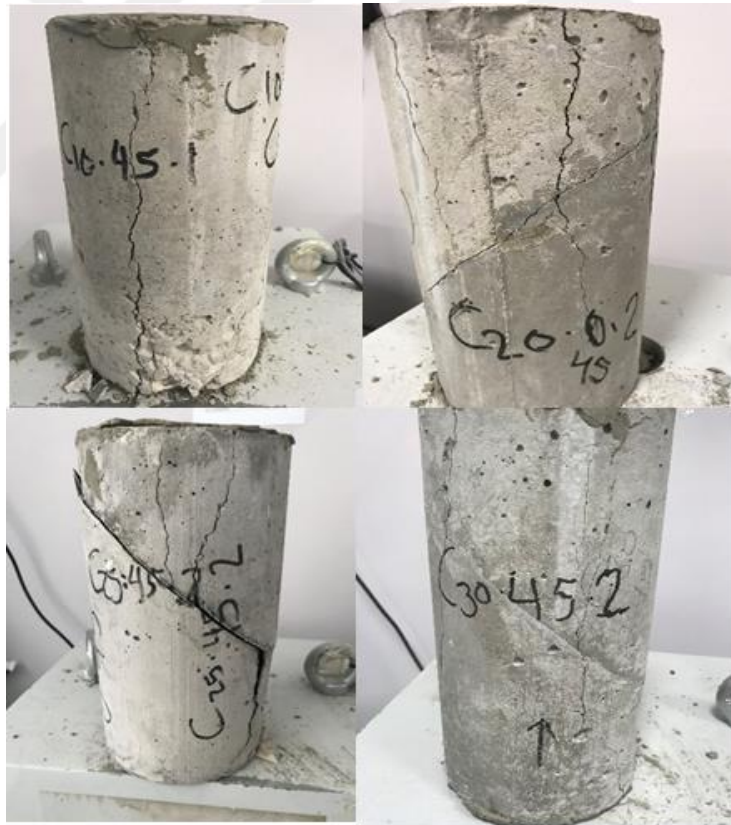
Figure 4.10. Compression test pictures of 45° cold joints.
