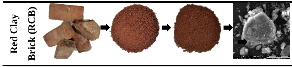
Figure 3.3. Red clay brick images (from left to right; raw state, crushed state, ground state, SEM micrograph)
