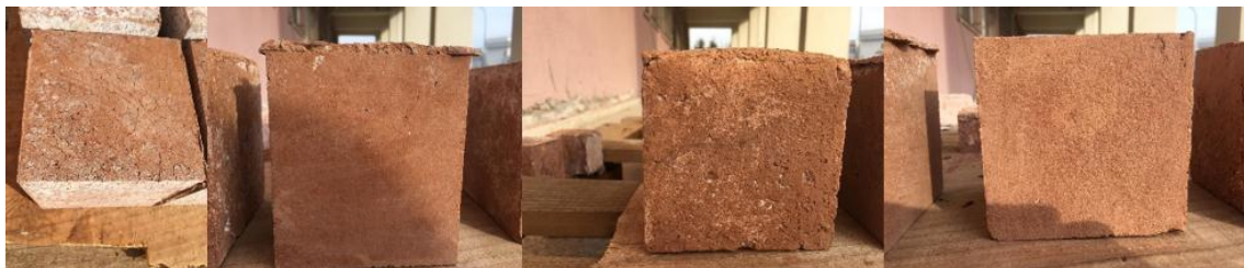
Figure 3.25. Geopolymer Concretes (the study carried out within the scope of the shrinkage behavior of the samples)
