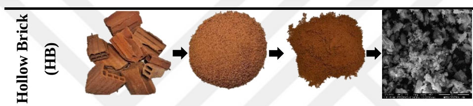
Figure 3.1. Hollow brick images (from left to right; raw state, crushed state, ground state, SEM micrograph).
