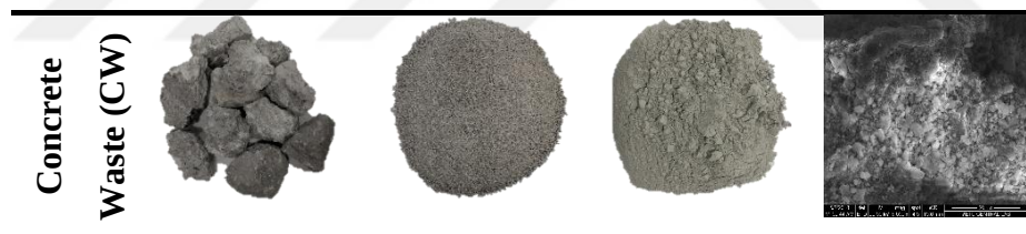
Figure 3.9. Concrete waste images (from left to right; raw state, crushed state, ground state, SEM micrograph)
