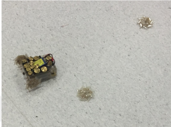
Figure 2.8: After a few runs, due to wear-out it detaches its wheels.
