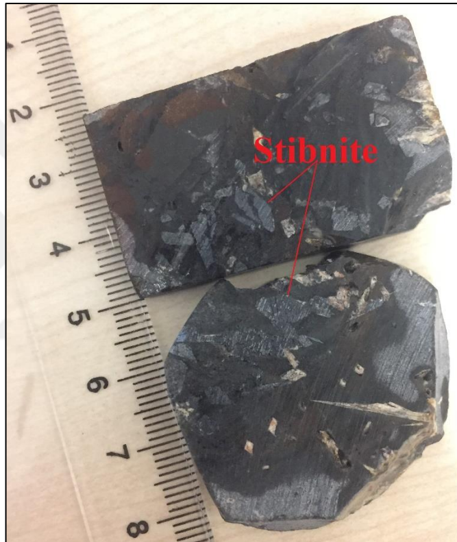
Figure 1.5. Stibnite crystals separated for sulfur isotope analyses collected from QSB-1.
