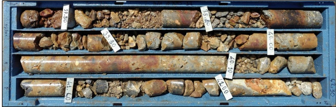
Figure 3.15. Matrix-supported breccia from 38.40 meters to 42.00 meters.
