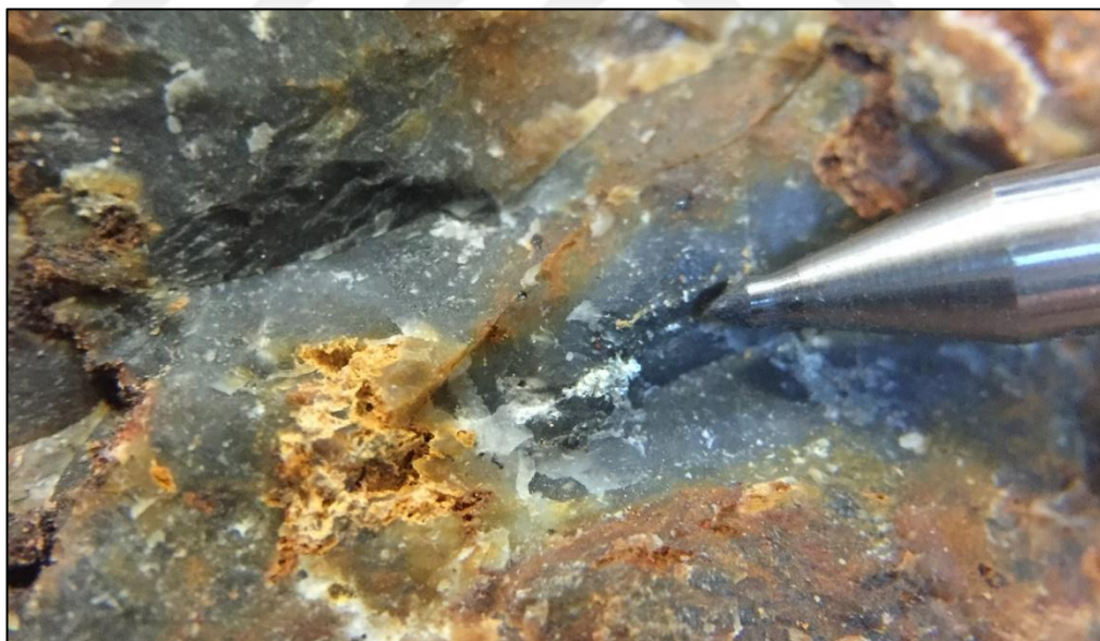
Figure 4.13. Arsenopyrite in pervasively silicified and strongly oxidized jasperoid
