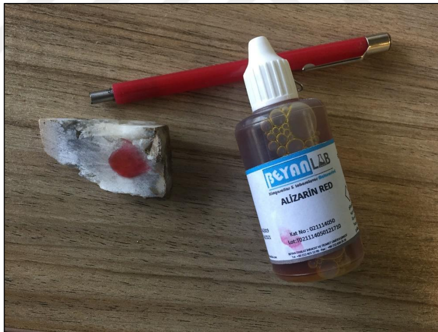
Figure 3.13. Alizarin red to test the composition of carbonate minerals at a sample from BLL.
