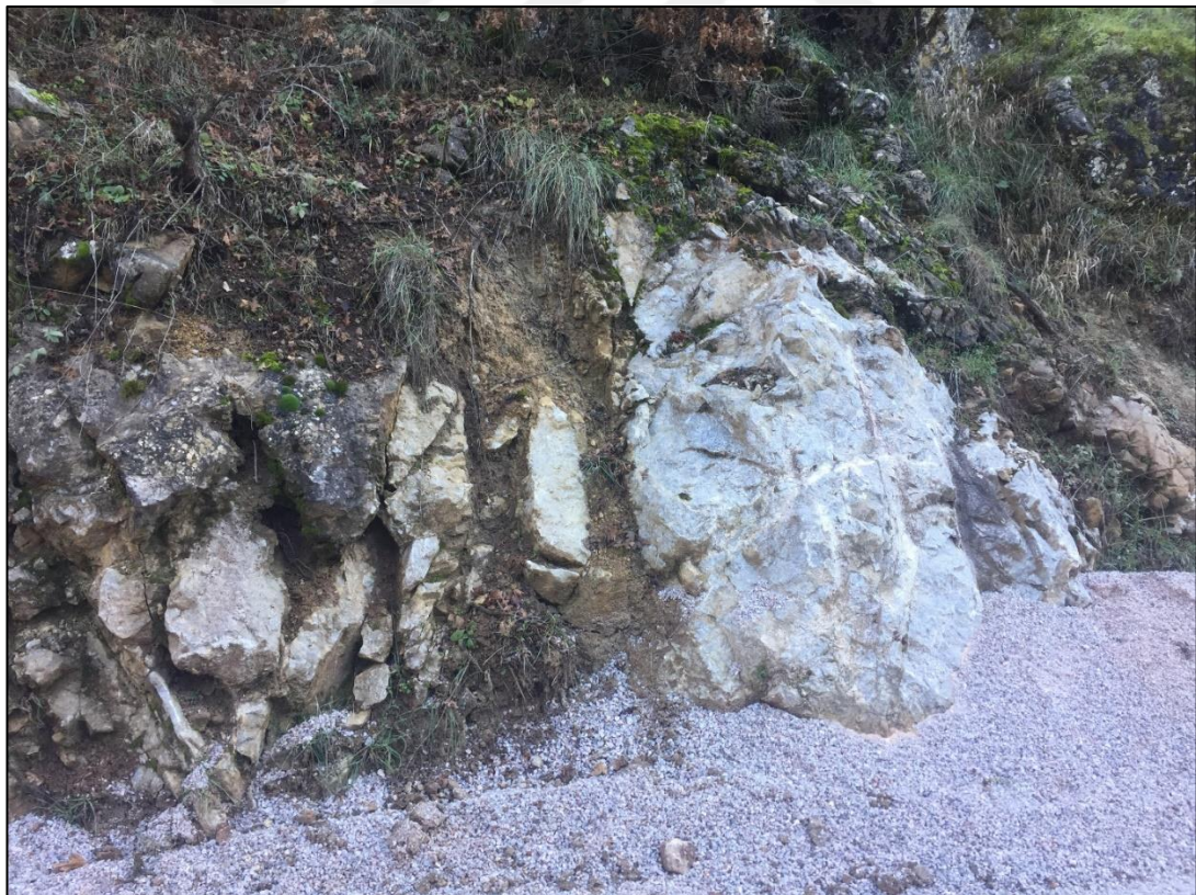
Figure 3.16. The field exposure of the light gray limestones traversed by calcite veins infilling the joint planes at the study area
