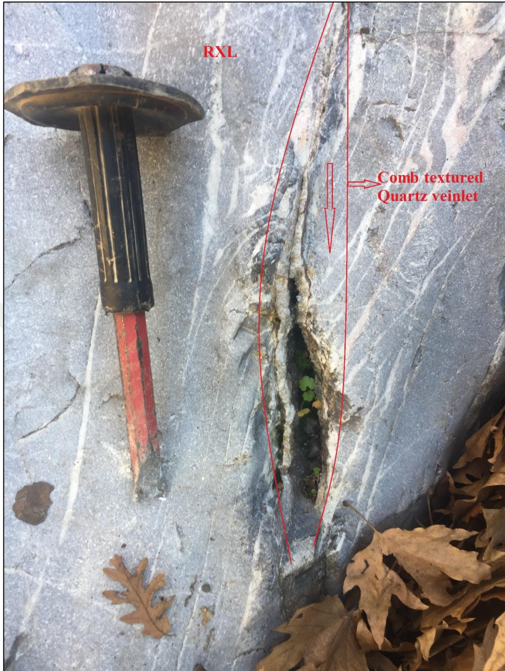
Figure 3.10. Comb textured quartz vein traversing dark-gray recrystallized limestone
