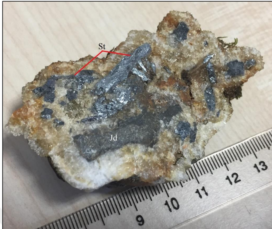
Figure 4.12. Sample with stibnite (st) and jasperoid (Jd) clasts in late (second phase) quartz
