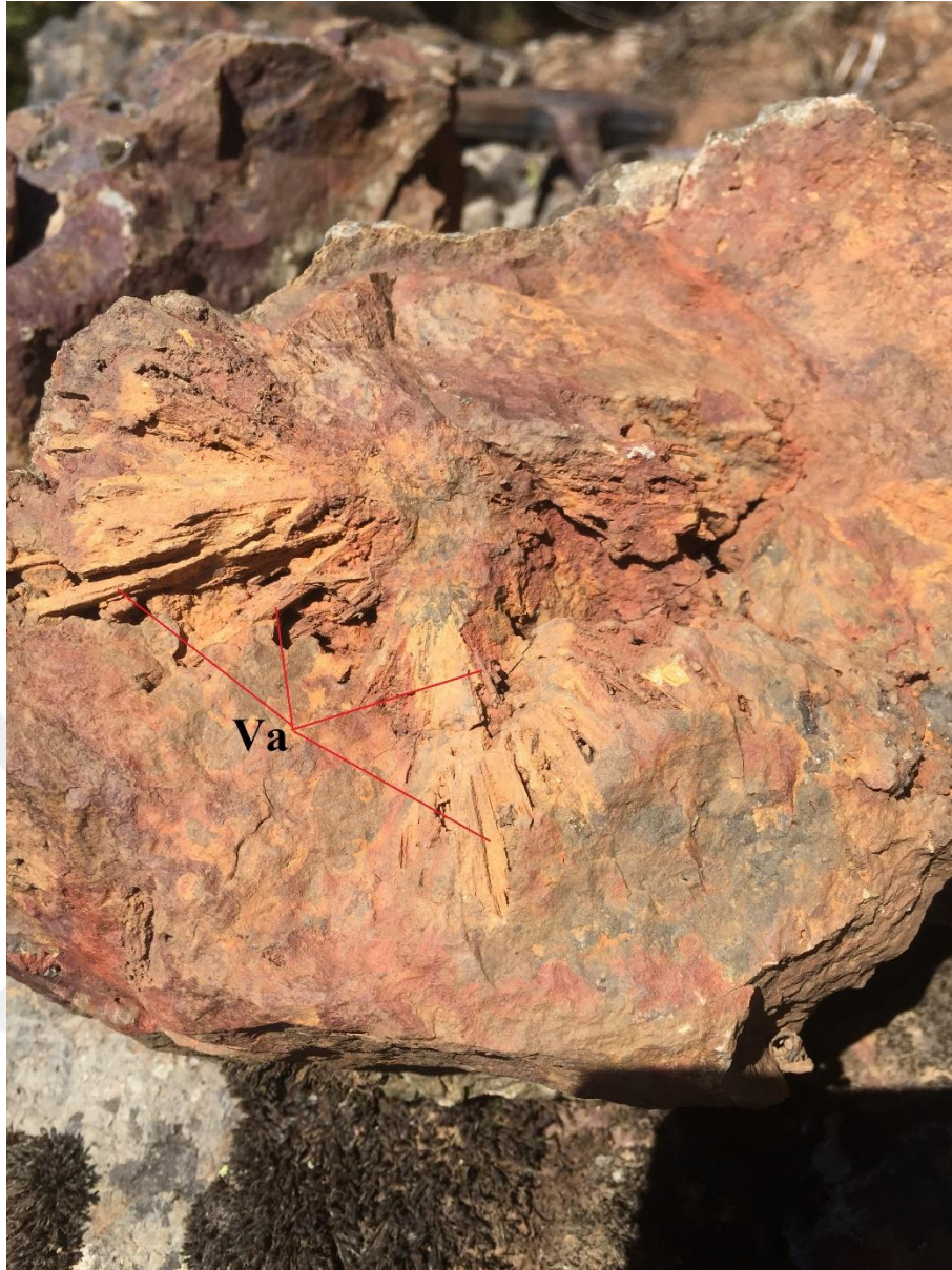
Figure 4.19. Strongly silicified and pervasively oxidized jasperoid includes valentinite (Va) which is oxidized mineral of stibnite (post-ore stage).
