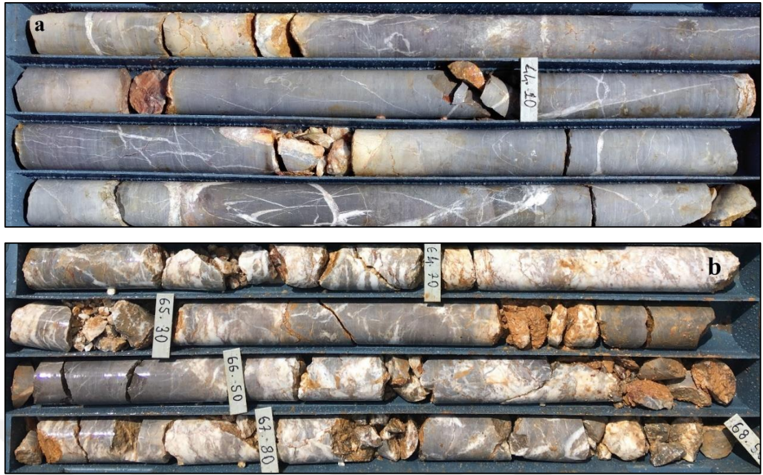
Figure 3.12. (a) Beige colored, laminated limestones and (b) stockworking calcite veins traversing the BLL, intersected at drill hole KTS-8
