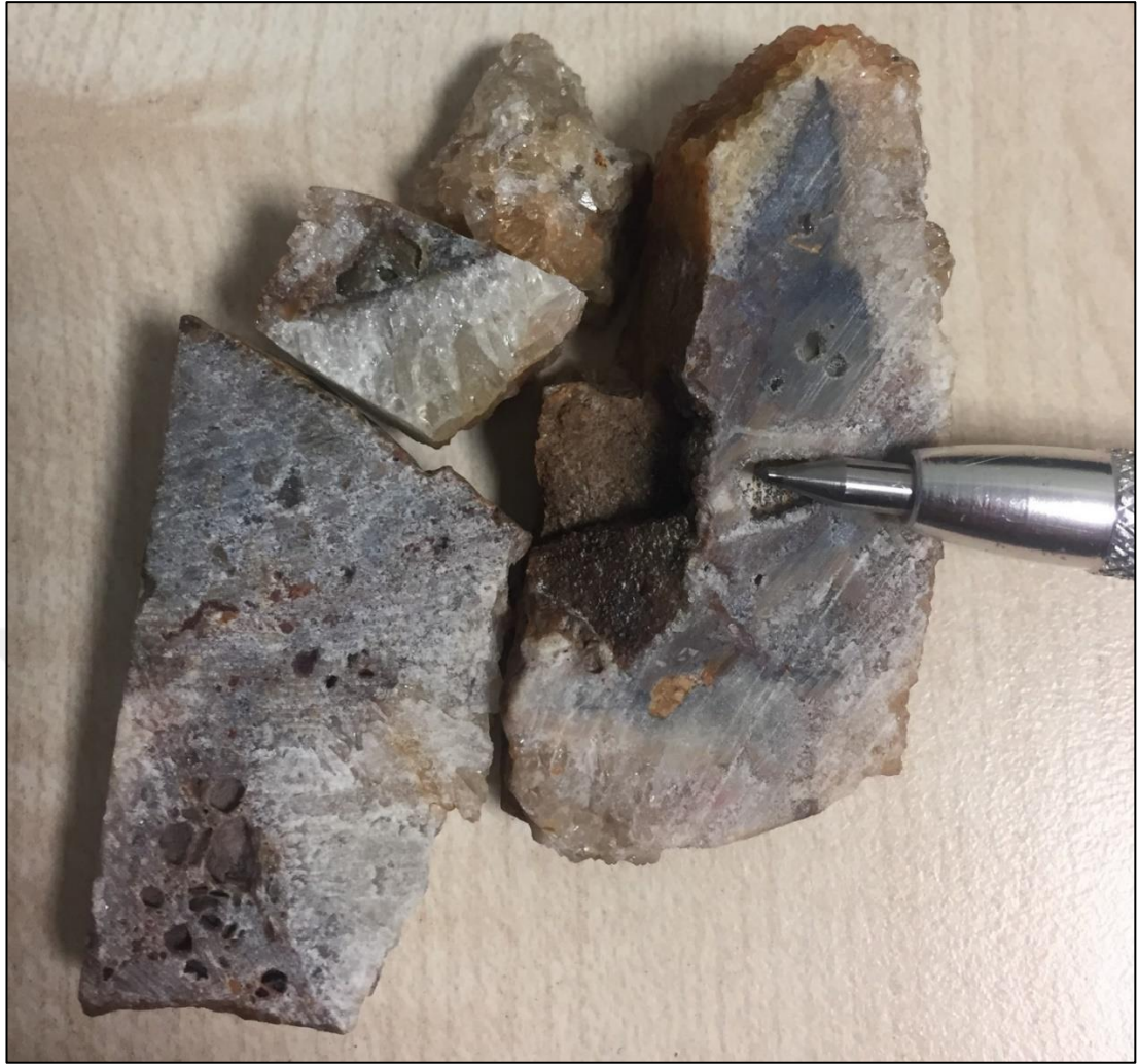
Figure 1.4. Q-1 sample syn-ore stage quartz veinlets included jasperoid
