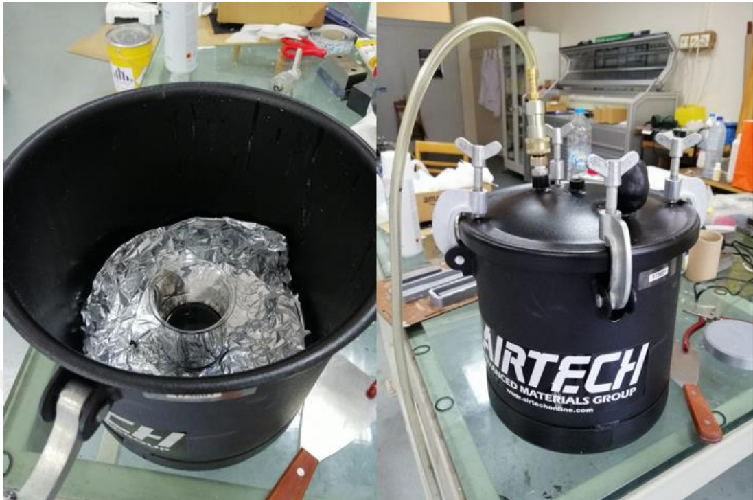
Figure 3.5. The nanoparticle incorporated epoxy system is kept in the Airtech vacuum chamber to eliminate the air bubbles.
