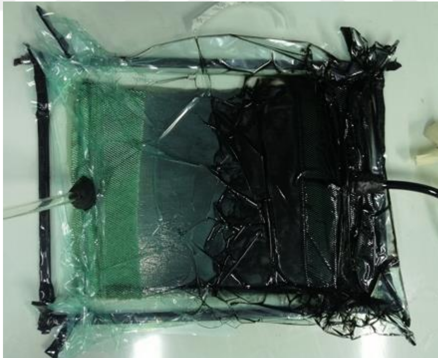
Figure 3.10. Accumulation of CNTs on the resin inlet side during vacuum infusion.
