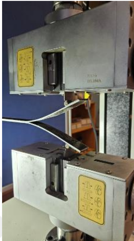
Figure 3.19. Test fixture to measure mode I interlaminar fracture toughness energy according to DIN EN 6033.
