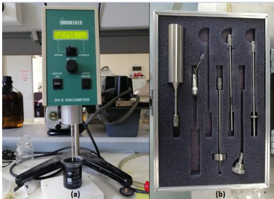
Figure 3.14. (a) Viscometer used in this study and (b) its spindles.
