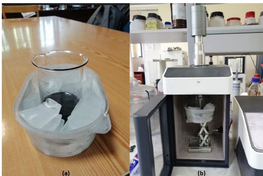
Figure 3.4. (a) The mixture was put into ice bath, and (b) placed in ultrasonic homogenizer.
