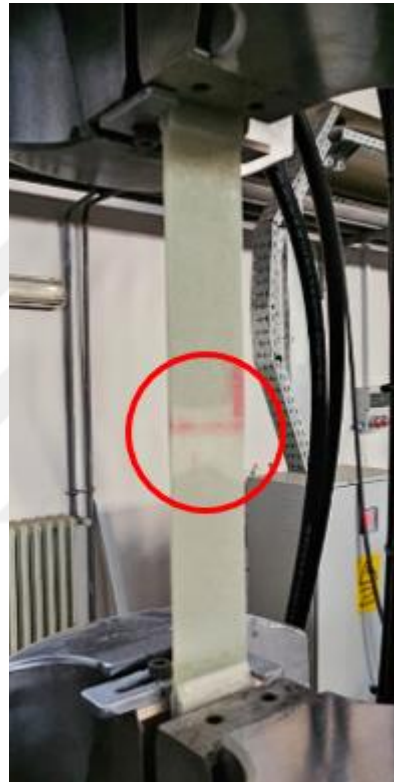
Figure 3.26. Delamination identification during the test.
