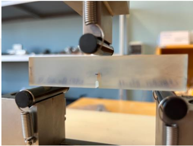
Figure 3.16. Fracture toughness specimen inside testing apparatus.
