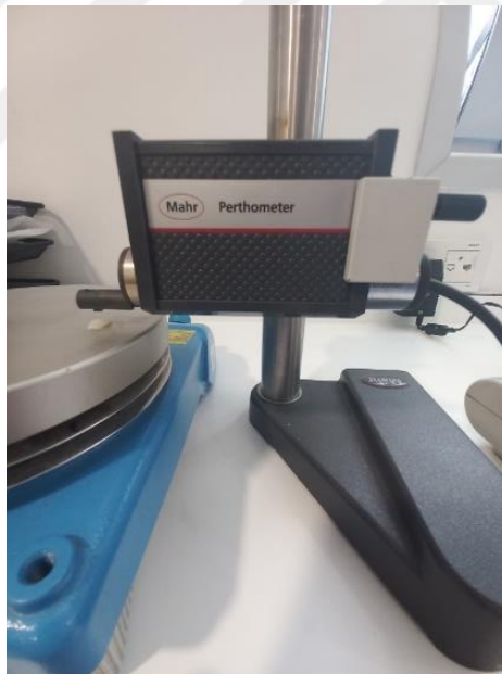
Figure 2.38. Measurement of surface of nonglazed Empress sample with profilometer device (Perthometer M1, Mahr)
