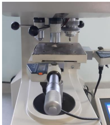
Figure 2.35. Microhardness tester, Buehler.
