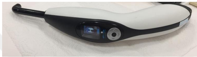
Figure 2.31. Polimerization unit for cerasmart samples (Ivoclar Vivadent Bluephase).
