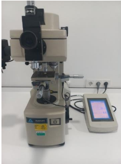
Figure 2.36. Microhardness tester (Buehler, Illinois USA).
