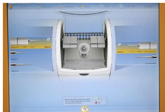
Figure 2.19. Selection of the burs before placing of the burs.
