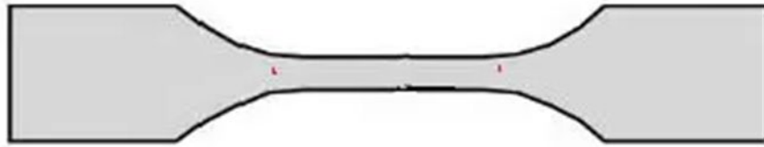
Figure 2.12 Standard dumbbell -shape specimens in tensile test
