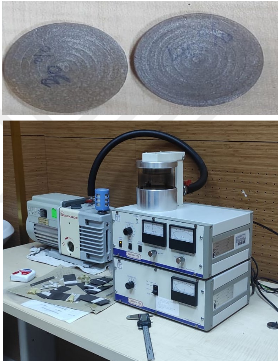
Figure 3.1 The coating machine and Samples of after coating
