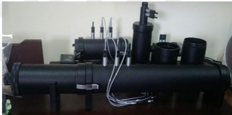
Figure 2.17 Two microphones impedance tube (Type Bruel-Kjaer 1406).
