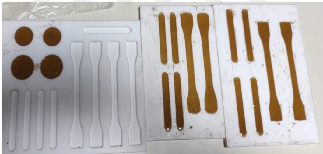
Figure 2.10 The specimens of polyester resin with filled PS powder
