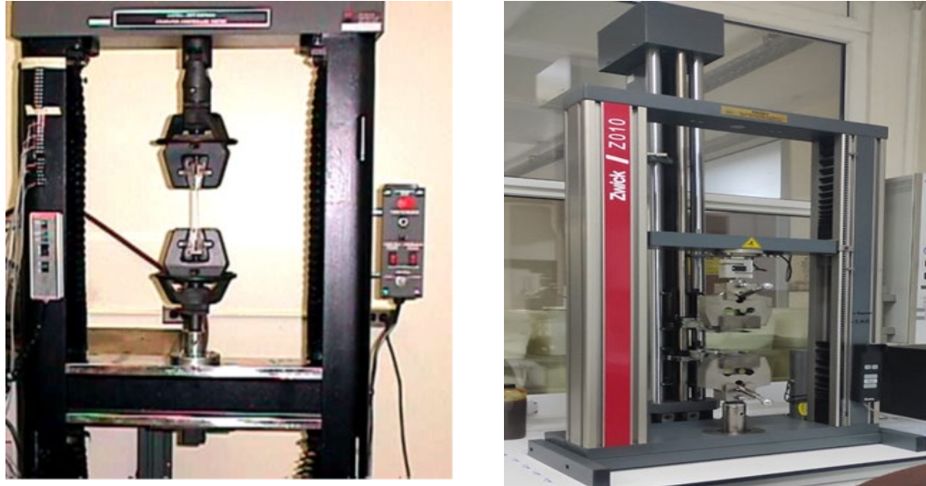
Figure 2.13 Tension test machine and specimen
