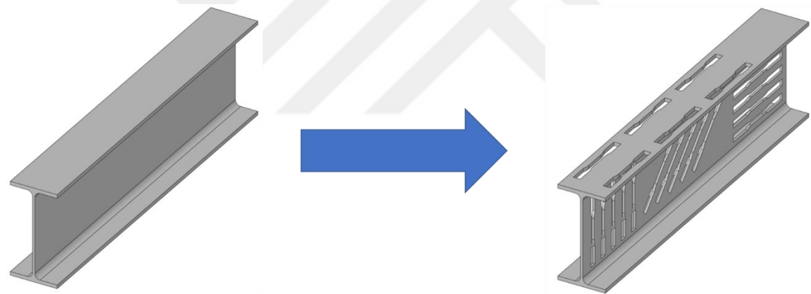
Figure 3.3. The demonstration of the manufacturing process applied for cutting the tensile specimens from an I-shaped beam.
