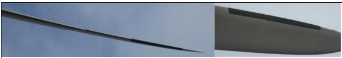
Figure 2.2. Roughness device employed on an actual wind turbine blade [59]
