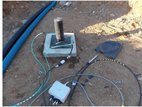
Figure 3.10. Hydraulic Settlement Device Placement in Derince Dam
