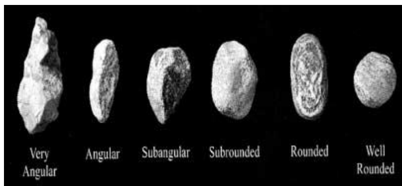
Figure 2.16. Categorization of Gravel Grain Shapes (Cudoto, 1999)
