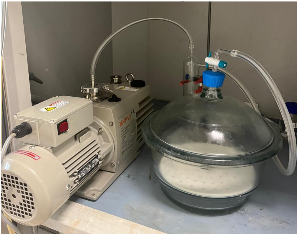
Figure 2.1: The setup for the vacuum-drying process. The desiccator (on the right), and the vacuum pump (on the left).
