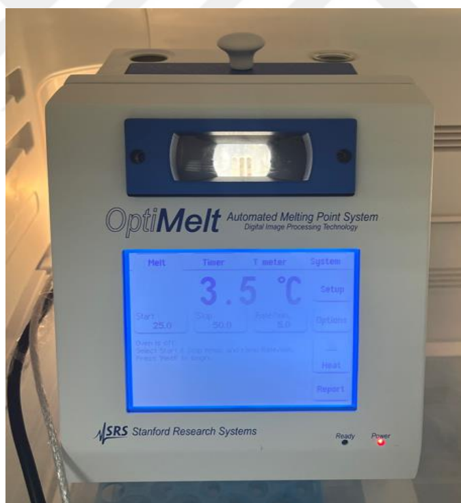
Figure 2.2: The Optimelt instrument, placed inside a refrigerator or freezer during the measurement.
