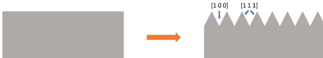
Figure 3.3: Surface modification with KOH solution to form a pyramidal textured surface.
