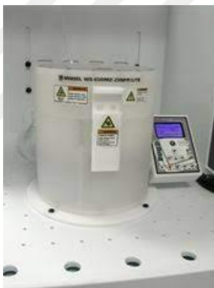
Figure 3.3. Laurell WS-650 model spin coater device.
