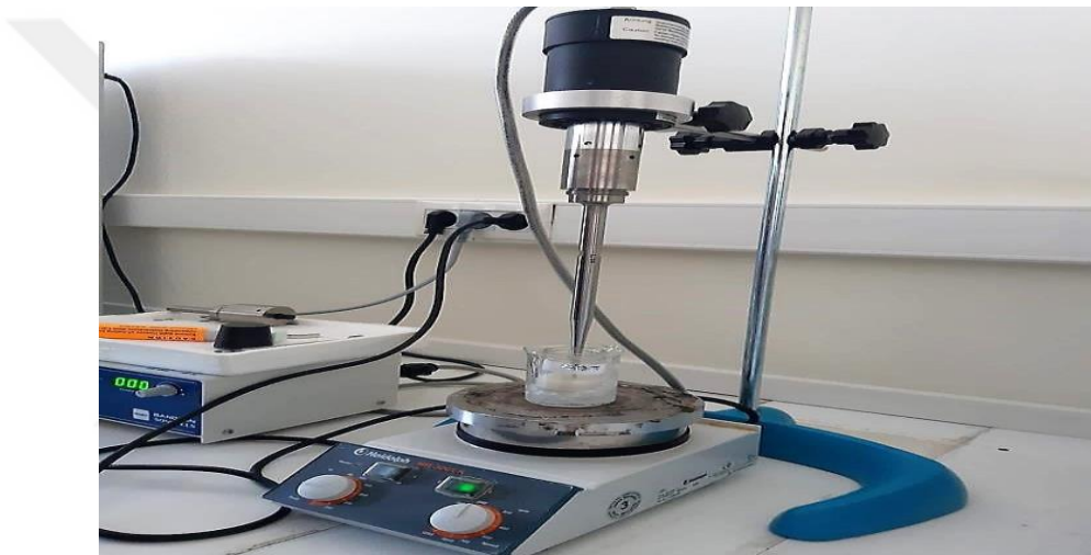
Figure 3.18: The sonication apparatus.
