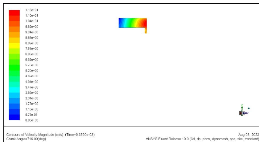
Figure 4.6: Velocity Contour at TDC at 2600 RPM.
