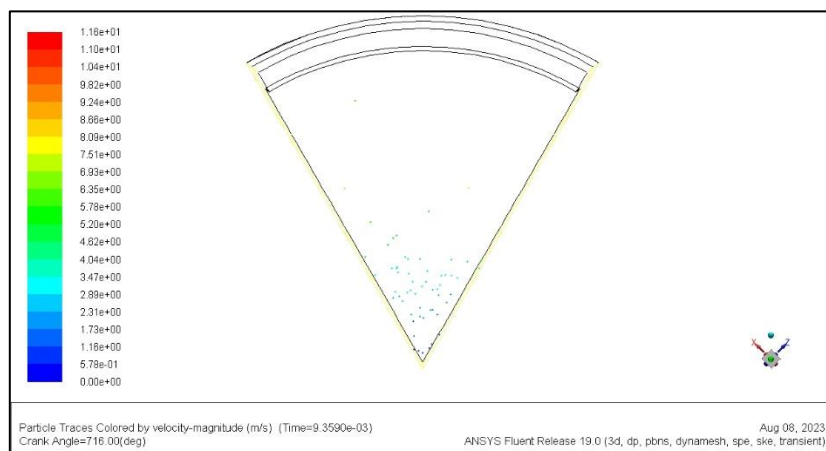
Figure 4.9: Particle Traces at TDC at 2600 RPM.
