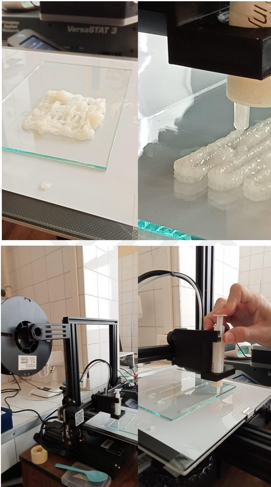
Figure 3.8 Process of 3D printing for hydrogels
