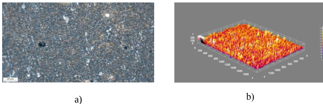
Figure 4.36 2 hours of He plasma processed anode Al pellet selected edge surface area Metallographic microscope image a) 500x magnification of the surface b) surface 3D graph generated by ImageJ software
