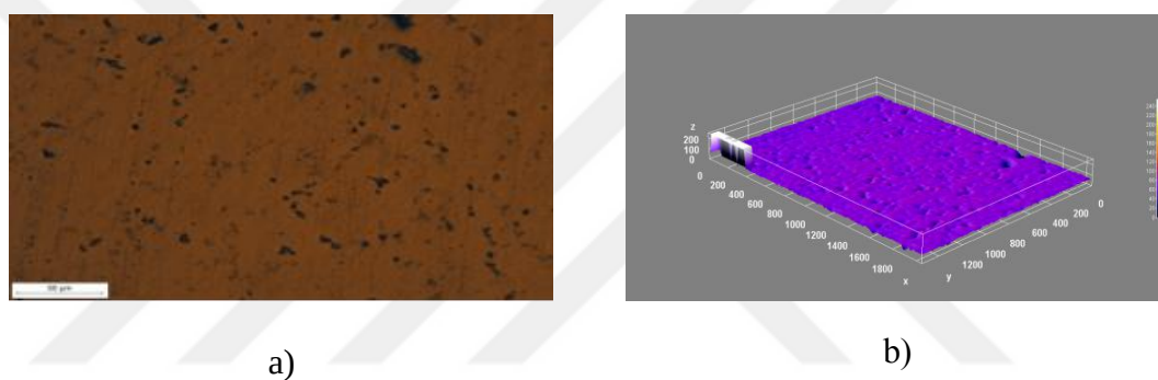
Figure 4.28 1 hours of He plasma processed Al pellet selected surface center area Metallographic microscope image a) 200x magnification of the surface b) surface 3D graph generated by ImageJ software
