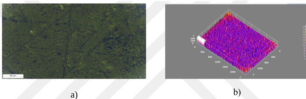
Figure 4.80 180 min time He plasma processed aluminum pellet anode surface without Metallographic microscope's light image a) 200x magnification of the surface b) surface 3D graph generated by ImageJ software
